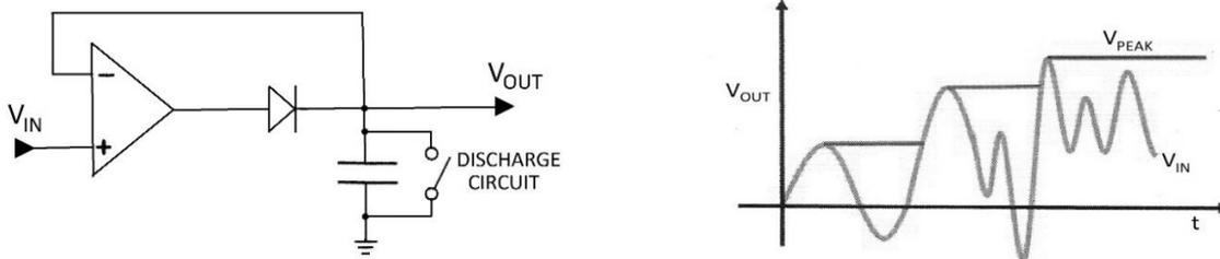
In an article titled *Peak Amplifier for an RF Wattmeter* Owen Duffy (VK1OD/VK2OMD) describes a practical generic amplifier circuit which would allow a conventional meter to measure the peak amplitude voltage of an SSB voice waveform. Similar circuits (with full details) are described in the RSGB publication *Test Equipment for the Radio Amateur*, 3<sup>rd</sup> Edition, §6.8 & §6.9.
